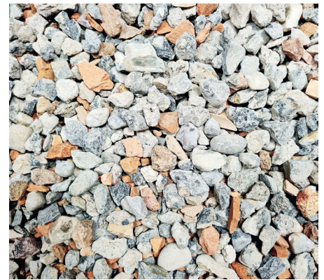
Type 2 recycled concrete aggregate: building rubble
