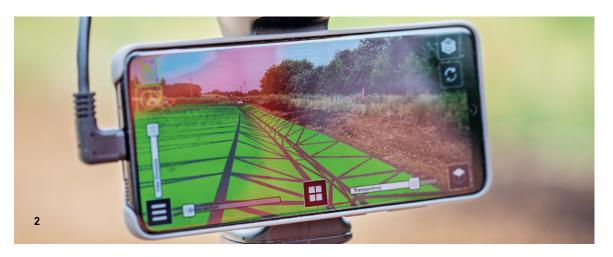
1 The BIM model always at hand: With mobile devices, the construction site staff can always consult the digital model. / 2 The smartphone superimposes the AR layer directly on the landscape, making the 3D data of the construction project visible.
