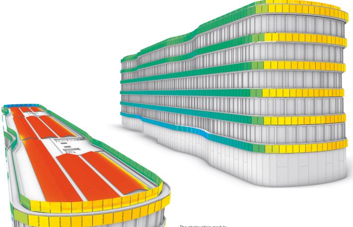
The photovoltaic module in GD ENERGY calculates the possible energy yields. Generative design
