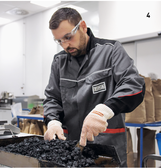
4 In the laboratory, the mixture with recycled asphalt is subjected to thorough testing. © Sebastian Sieberer
