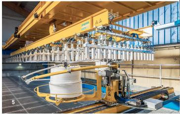
4 The formwork robot places the formwork precisely where it is marked on the plan. /
